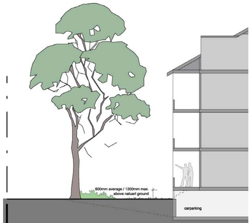
Figure 14: Basement car parking protruding above natural ground level
