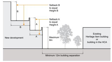
Figure 19D.2-1: Building separation requirements for development greater than 8m high (2 levels) within a Heritage Item site.
