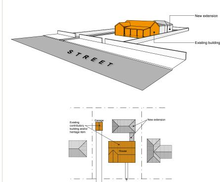
Figure 19D.5-2: Retain original doors and windows to front and side elevations (coloured orange) of heritage items.
