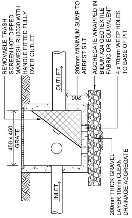
**SITE DISCHARGE AND SILT ARRESTOR PIT (450 x 450)**
