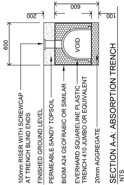
SECTION A-A: ABSORPTION TRENCH
